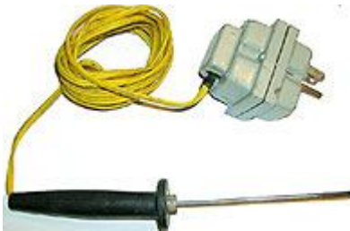
Western Electric 945A1 Tool s/n 7057 for crimping 710 splices from Chuck Hensley
