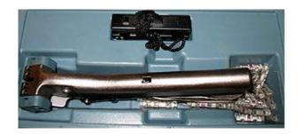
CMC 5334-A - The CMC 5334 Polar Probe is a test pick used for determining the presence of various voltages when testing equipment for trouble conditions. It detects battery, ground, ringing generator and may be used on dry reed relays and all types of solid State Circuitry.
