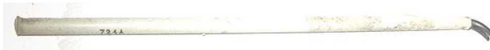
Bell System - Number not currently known - tool to punch a hole in the sheath of lead cable for insertion of an air fitting.
