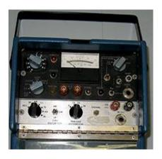
Atlantic Research DATA TECH DTS-1-M470/483 teletype loop tester: There is a built-in FOX generator (the Quick Brown Fox Jumped over the lazy red dog - which tests all characters on a terminal), that will do baudot, ASCII, Teletypesetter, and EBCDIC, and a built in distortion analyzer.
