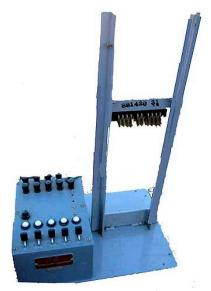
AE Linefinder Test Stand H - 85829-1-2 - used for testing Strowger linefinder switches.
