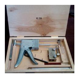
The kit was made for replacing coils of NE-AF, NE-AG, NE-AJ, and NE-AK type relays. (line and cutoff type). A BSP for the use of this kit maybe found on the TCI document library, 040-272-801.
