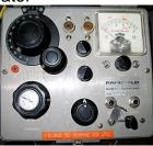
43-114 - Radio Shack in-store telephone tester, test dial tone, dial, loop, cords, Tx and Rx, etc.
