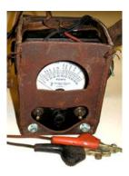
KS-21250 L1 Coin Crafts Test Set - Checks payphone coin relay, sidetone, Refund/Collect Function, etc.
