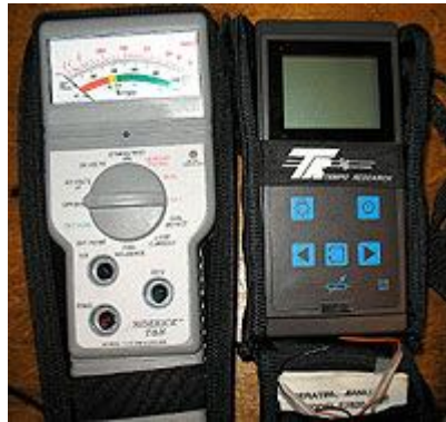
Tempo Sidekick T&N (left) - same as 7B plus 5 additional measurements Tempo E2520 TDR (right) - TDR for display of line faults and graphical display, line measurements.
