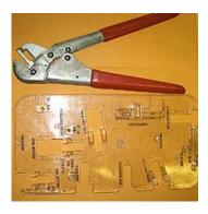
799 - Notching Template - used to guide installers to place notches in the correct position when using the 798A tool.
