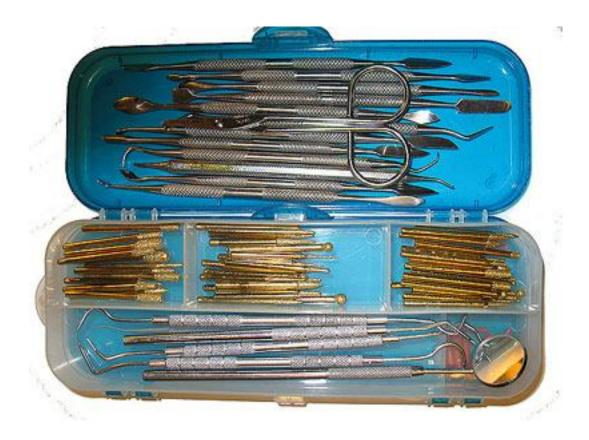
Assorted Dental tools used for a number of purposes. Picks are used to remove solder from PCB boards, spatulas for repairing plastic and bakelite cases, mirror for viewing under boards, titanium/diamond burrs and drills to grind and repair cases, hemostat for holding wires while soldering. All are contained in a cheap pencil box from the dollar store.
