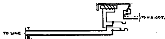
Line Circuit No. 1240-D Switchboard
